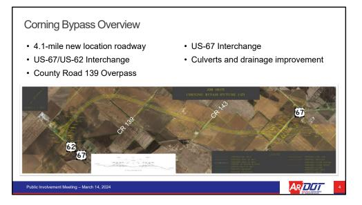
The 4.1-mile Corning Bypass would extend north from an interchange with Highway 62/67, approximately 2.7-miles west of Corning, and terminate approximately 2.5-miles north of Corning at an interchange with Highway 67. The bypass would be a fully-controlled access facility designed to interstate standards.
