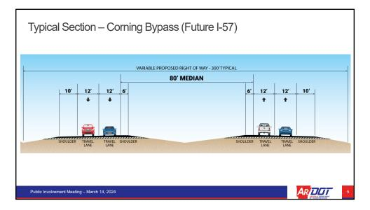
The typical section for the Corning Bypass will be a four-lane divided highway with a depressed 80-foot-wide median and an approximately 300-foot-wide right-of-way. The roadway will have four 12-foot-wide driving lanes with 6-foot-wide inside shoulders and 10-foot-wide outside shoulders.
