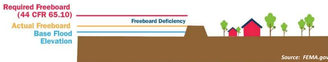
Figure 58: Example of a Levee that has a Freeboard Deficiency
