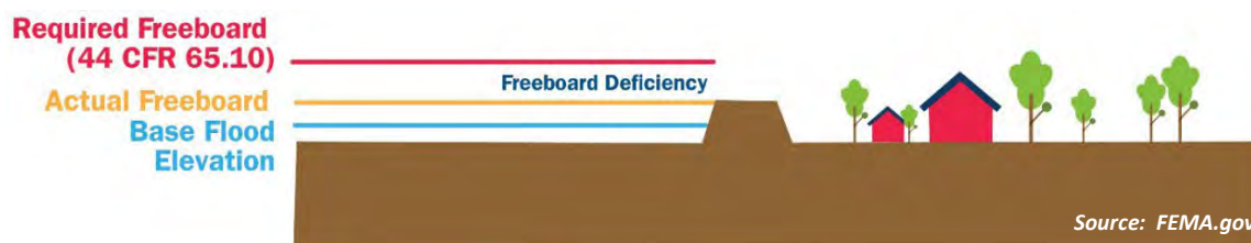
Figure 7: Example of a Levee that has a Freeboard Deficiency
